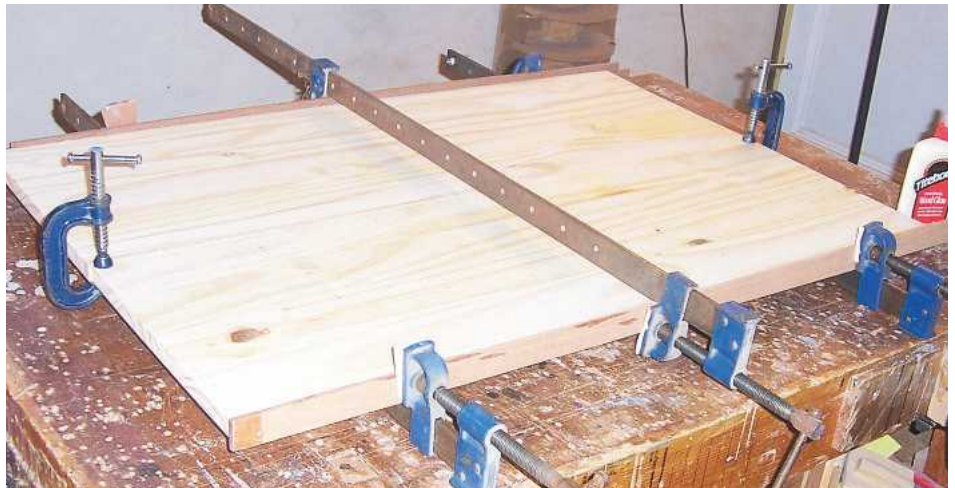
▲ Pic.2 Sash cramps are used to achieve the butt joint in the boards
